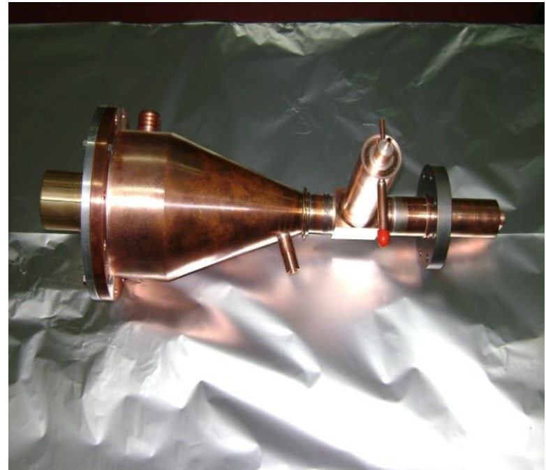
Coaxial coupler assembly after brazing
