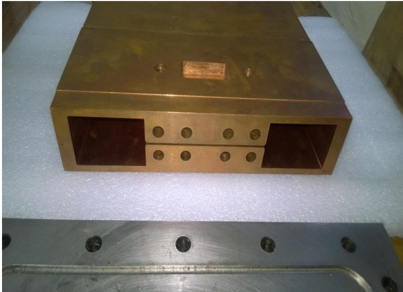
Two copper halves and S/steel flange before brazing
