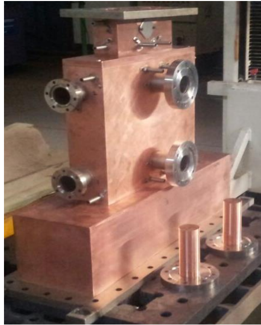
250 kW CW, 352.2 MHz Waveguide Coupler for LEHIPA
