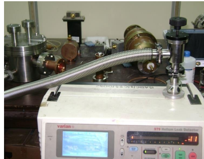
RF Coupler leak tested at LEHIPA, BARC
