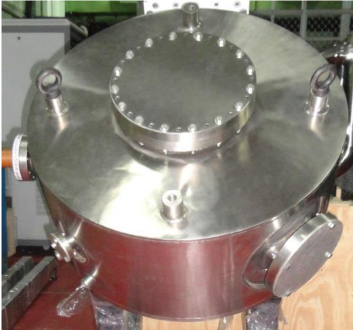
Test cavity for 250 kW, 352.2 MHz Waveguide Couplers
