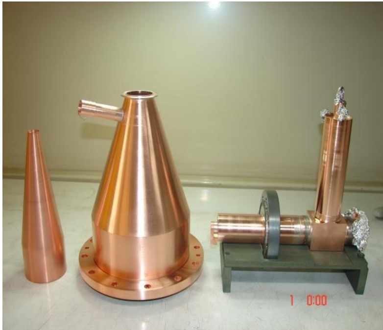
Coaxial Coupler parts before brazing of final assembly
