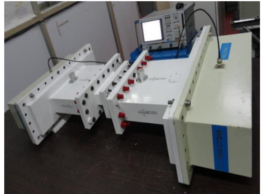
250 kW, 352.2 MHz ridge loaded waveguide iris coupler prototypes for RFQ and DTL cavities
