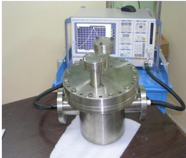
RF Cavity developed for Coaxial Coupler Conditioning
